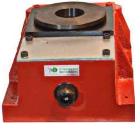
VHS Festofix Leveling Wedge Mounts are useful in leveling and aligning machinery to very strict tolerances and make it possible to vary adjustments at any time, even under maximum loads requiring only a small hand wrench to adjust. These mounts provide the most rigid machine-to-foundation connection. The 3-piece wedge design provides true vertical lift and eliminates lateral movement as machines are raised or lowered.
