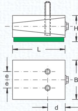
Dynemech's DTH Series mounts are designed for machines which require very high height adjustment and precision levelling. Variations are available for free standing and bolt on machine bases either with or without insulation damping. Dynemech also provides tailor made solutions besides providing quick installation service.
