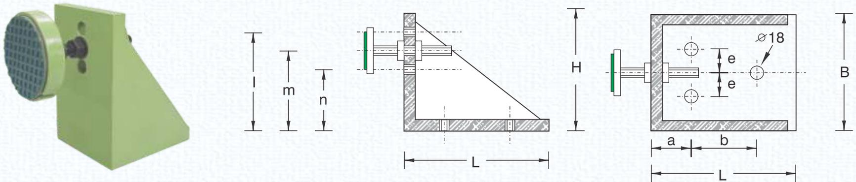
**Dynemech Horizontal Stop Series DHS** is suitable for the shock absorption of machines having very high axial force on a light weight machine bed and for precision machines which has to be flexibly mounted but be protected from horizontal shaking due to inherent axial movements of their elements.
